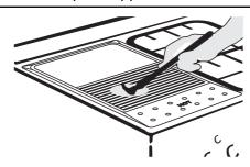
Position the griddle over the hotplate burners resting on the pan support. The griddle can be lightly brushed with cooking oil before use. Light the hotplate burners. Adjust the flame heights to suit.
